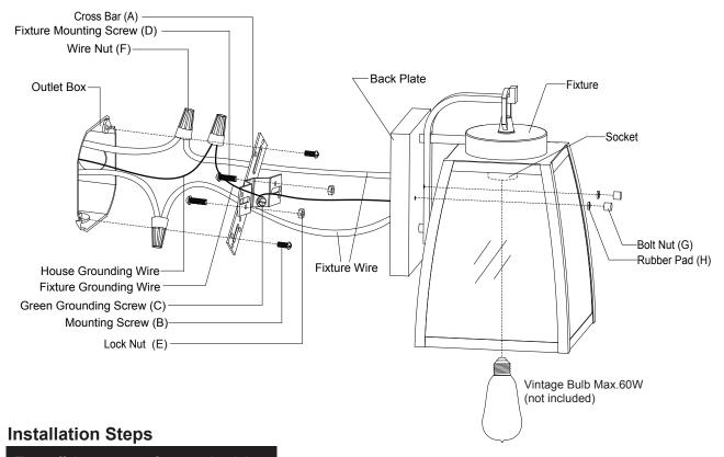
Turn off the power at fuse or circuit box.
