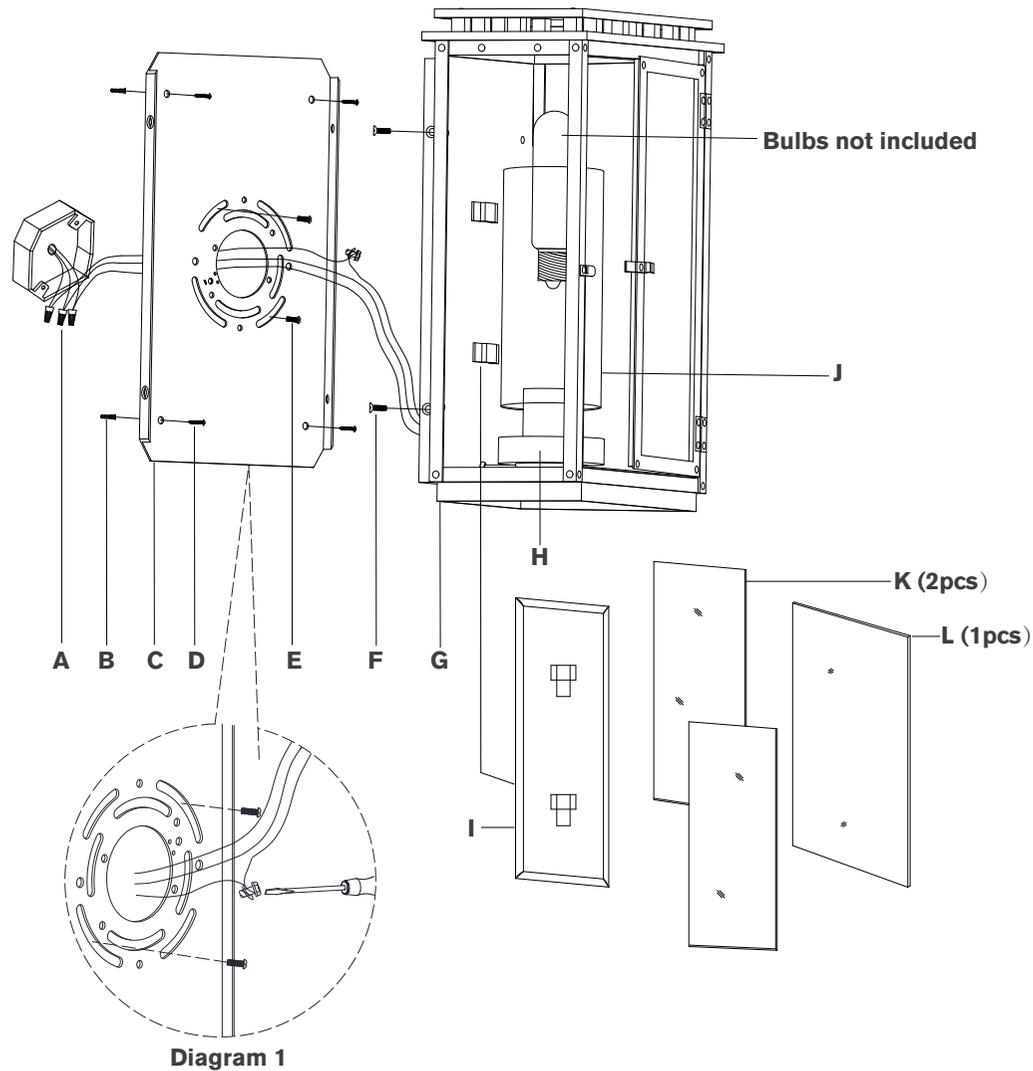
11. Open the door, Install glass panels **(K)** to the side of fixture frame **(G)** and secure it by bending metal tabs.
